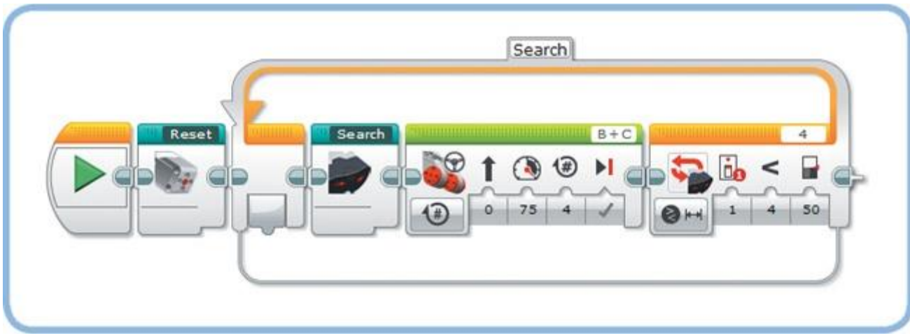
Figure 18-19. Step 1: The robot searches for the beacon until it's nearby.
