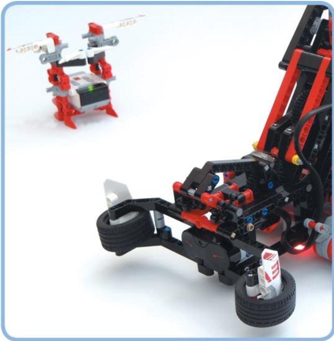
Figure 18-18. Place the IR bug about 1 meter (3 feet) away from the robot. The robot can face in any direction, but the beacon should point toward the robot.
