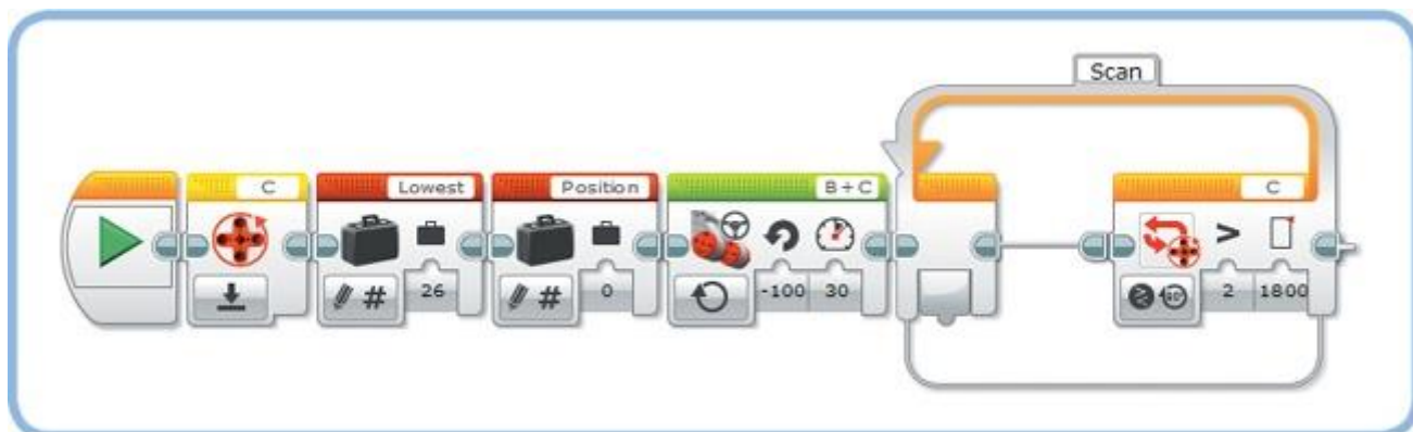
Figure 18-11. The search algorithm. The Reading variable contains the absolute value of the Beacon Heading and is considered valid if it isn't 0.
