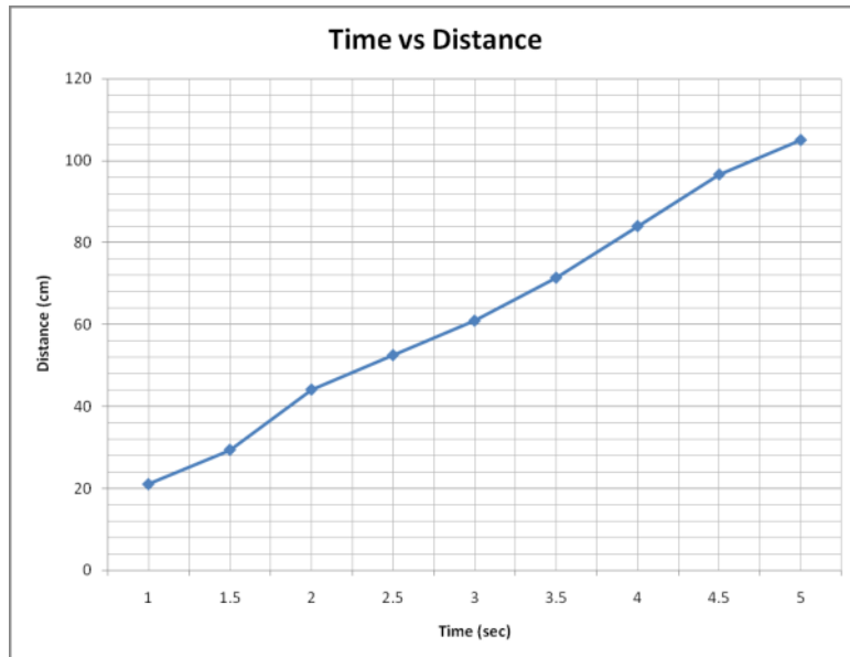
Fig 5. Distance travelled by the robot, as a function of the time travelled
