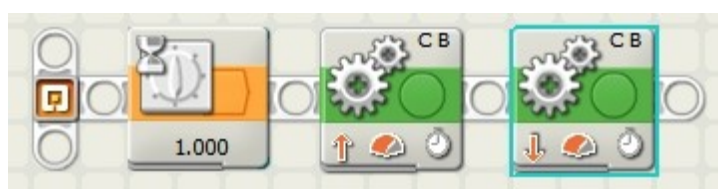
Fig 9. Complete Mexican Wave program. Each robot waits a pre-determined time, and then travels forward 1 second and backward 1 second.
